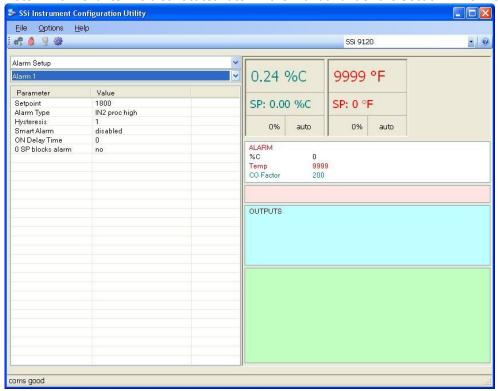
The 9120 controller can be configured to use three different alarms. Each of the alarms consists of an alarm setpoint, alarm type, alarm hysteresis, smart alarm, ON delay time, and a 0 SP blocks alarm value. The alarms come from the factory with a default configuration dependent on the application but also can be modified prior to shipment to your facility or in the field by a supervisor.
