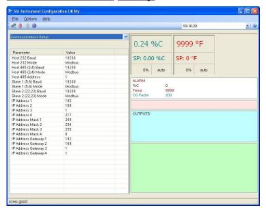
*Communications Setup* is the communications definitions for the controller. Please contact Super Systems Inc. at 800-666-4330 for more information regarding port setup. It is *strongly recommended* that none of the settings be modified
