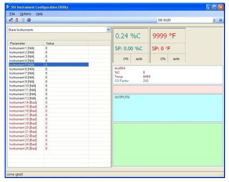
This value is a display of the minimum millivolts measured during the last burnoff.
