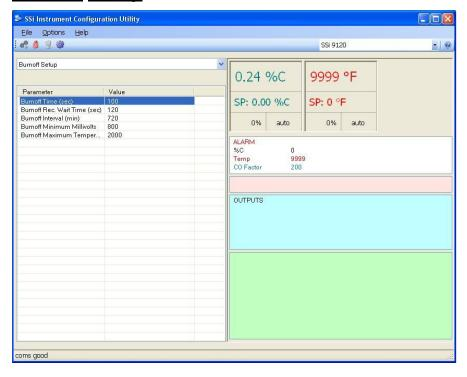
This menu option allows the user to modify the settings that are associated with the probe burnoff (menu option *Burnoff*).
