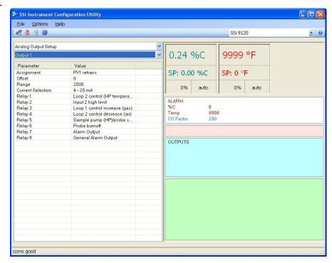
Clicking on this value will display an input box, and then you can use the pull-down menu to select the desired parameter. Once selected click **OK** and the displayed assignment under Value will be the current assignment type. The following is a list of the options:
