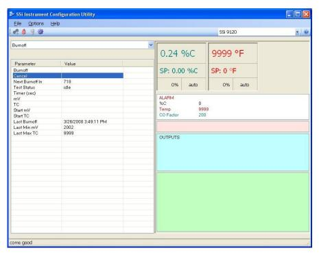
When a probe is in a furnace, soot will collect in the end of the probe, which will have a negative effect on the performance of the probe. Burnoffs are used to clean out the built-up carbon by burning it off of the probe. To manually begin a burnoff, click on the "Value" area next to "Burnoff". To Cancel a burnoff, click on the "Value" area next to "Cancel". Note: "Burnoff" and "Cancel" are the only two interactive fields on this screen; the rest are read-only.
