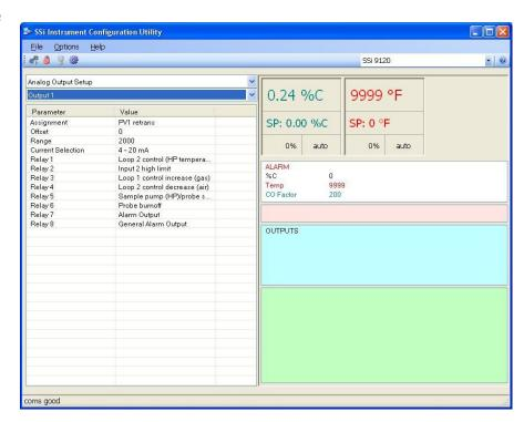
two analog outputs. The outputs are ranged for a 4-20 milliamp signal or a 0-20 milliamp signal. Each output comes with a factory default configuration dependent on the application. Each output can be modified prior to shipment to your facility or in the field by a supervisor.
