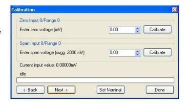
value for the input. Press the **Back** button to return to the previous screen or press the **Next** button to view the next screen. The **Set Nominal** button will set nominal values for the inputs. Press the **Done** button to close the calibration screen down.
