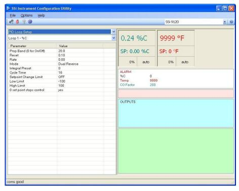
PID is the tuning parameters entered for each Process Variable loop. The loop value can be either **Loop 1**, or **Loop 2**.
