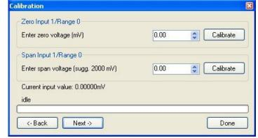
the previous screen or press the **Next** button to view the next screen. Press the **Done** button to close the calibration screen down.
