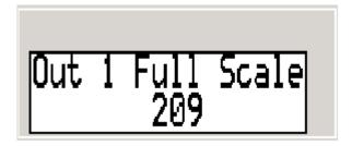
The valid range of values for output 1 full scale is zero to nine thousand nine hundred ninety nine. To change the value, press the up arrow key once so that the rightmost number begins to blink. Pressing the up arrow again will increment the value. Pressing the **NEXT** key will display the next screen, *Output 2 Full Scale*. Pressing the **PREV** key will display the previous screen, *Output 2 Exponent*.
