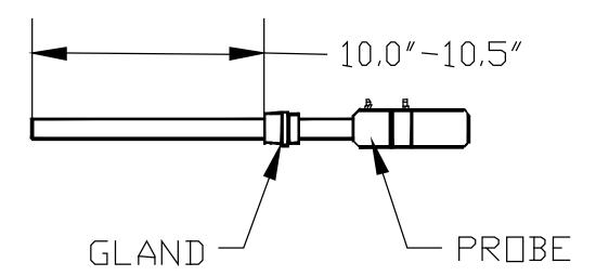
Once the probe has been inserted into the heater, make the necessary electrical connections at the head of the probe. The green thermocouple wire from the electrical enclosure box should be attached to the thermocouple connection at the head of the probe (Positive (+) = Black and Negative (-) = Red). The sensor wire should also be attached to the probe (Positive (+) = Black and Negative (-) = White).
