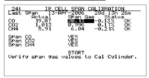
The IR Cell Span Calibration page is used to span calibrate the IR cells. It is very important to be sure that a Certified Primary Standard sample gas within the noted specifications is used. The nominal composition of this gas should be: 20% CO (Carbon Monoxide) 1% CO2 (Carbon Dioxide) 6% CH4 (Methane or Natural Gas) 40% H2 (Hydrogen) Balance N2 (Nitrogen) When viewing this screen, the
