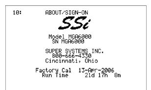
This page is the sign-on screen that shows the SSi logo and phone number. Also shown is the unit serial number, the date of the last factory calibration, and the number of days, hours, and minutes that the instrument has been in use since the last factory calibration.
