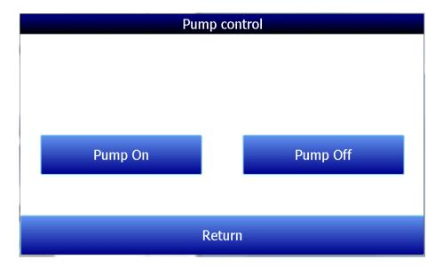
Pump Control will allow the operator to turn the pump on or off by selecting the corresponding button. Pressing **Return** will display the Menu list.
