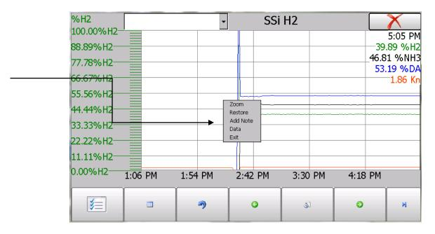
The **Zoom** option will allow the user to zoom in on a particular part of the screen. Once this has been selected, the user can take a stylus or a finger and create a box around the desired data. Once the user releases the stylus or finger, a zoom is no longer possible, and the user will need to re-select the option from the sub-menu to zoom in again.
