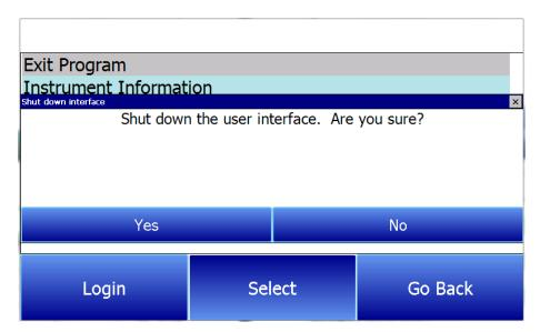
Selecting Exit Program will allow the operator to shut down the user interface. This can be done by selecting **Yes** when prompted or **No** to return to the Menu list. If the user interface is shut down, it will restart automatically when the power to the instrument is cycled.
