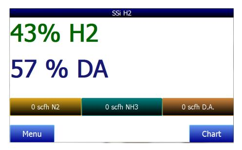
The home screen also displays the flow of  $N_2$ ,  $NH_3$ , and D.A. These values can be entered by the operator when the instrument is in the mode to evaluate Kn or %DA. This is discussed further under the Instrument Configuration section. The **Menu** button in the bottom left-hand corner will take the operator to the configurable options within the controller. The **Chart** button in the bottom right-hand corner of the screen will display the data trend chart.
