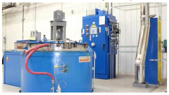
Our goal is to provide you with the right equipment for your atmosphere control needs, whether it be carburising, nitriding, ferritic nitro-carburising or any other process using atmosphere measurement and control.
